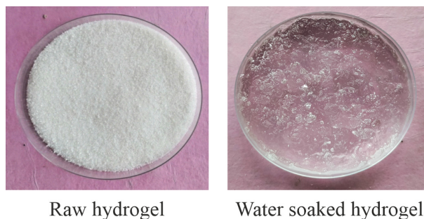
Fig. 2. Status of raw and water-soaked hydrogel
