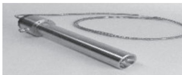
Fig. 4. Frequency domain reflectance (FDR) probe for soil MC measurement
