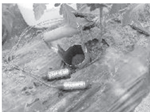
Fig. 2. Soil Electrical Resistivity (ER) or Electrical Conductivity (EC) probe near a plant for installation
